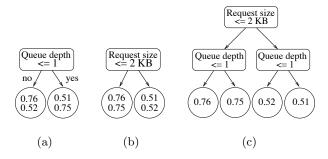
Figure 3: An example of the steps taken by CART in building a regression tree from the samples in Table 3. CART determines which split is "best" by inspecting the similarity of the samples in the leaf nodes. In this example, option b (request size) is a better first split than option a (queue depth). For the next split, CART then selects the queue depth.
