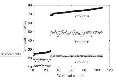
Figure 6: Device similarity. The performance of each array changes similarly, indicating that the performance of one array is a good predictor of another.
