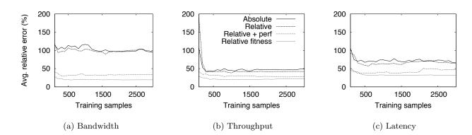
Figure 9: Accuracy versus number of training samples. The top line represents the absolute model, the next line is a relative model that captures changes in the workload characteristics. The third line is a relative model trained with performance. The fourth line (least error) is relative fitness. As the number of training samples increases, the relative fitness models are the most stable and also the most accurate.
