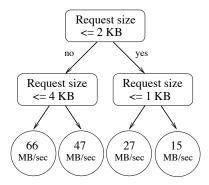
Figure 2: A regression tree that learns the performance of a disk drive for sequentially-read data.
